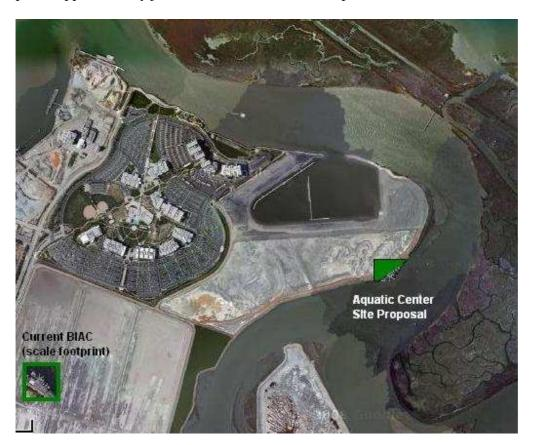
This proposed location has reasonable tidal water access, protection from prevalent northwest winds, and does not require incursion into sensitive habitat. Approximately two acres are suggested to allow space for adequate parking, fire access, a 4800 sq footprint boathouse, outside boat shell storage racks, ramp access to docks, and open transit and work corridors. A workable layout might look like this:
